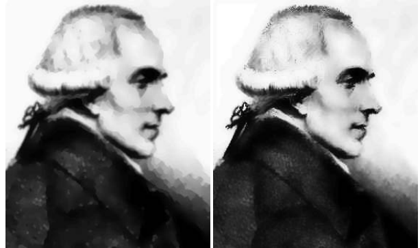
Figure 2: Edge-preserving smoothing: anisotropic diffusion with 20 time-steps of \tau = 1.0 (left) and Gaussian bilateral filtering with a 30 \times 30 window size, \sigma_D = 5.0 and \sigma_R = 30.0 (right). \sigma_D and \sigma_R are bilateral filtering parameters, see [6] for details.
